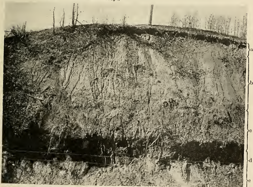
FIG. 45.—A section showing (a) Bloomington gravel; (b) Shelbyville till sheet; (c) Iowan loess; (d) Sangamon soil; (e) Silt below peat. (Dr. Samuel Calvin, U. S. Geol. Survey.)
